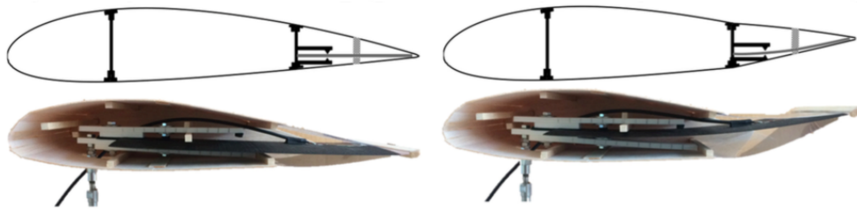
Figure 2.3: Concept of a passively morphing wing flaperon by means of an embedded bistable composite plate proposed by Nicassio et al. [121].
