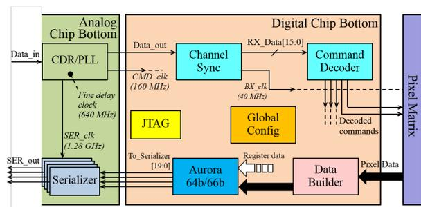
**Figure 3:** Block diagram of RD53A digital chip bottom.
