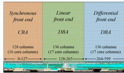
**Figure 2:** Arrangement of analog FE flavors and digital buffering architectures in RD53A layout.
