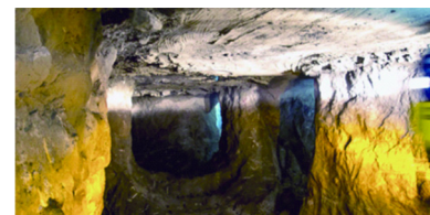
Fig. 15. Quarry site analyzed and the room-pillars system is clearly noticeable.
