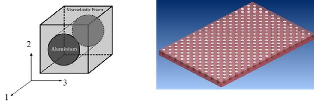
Figure 1: A sketch representation of an acoustic metamaterial unit cell and a view of a numerical model of a metamaterial panel.
