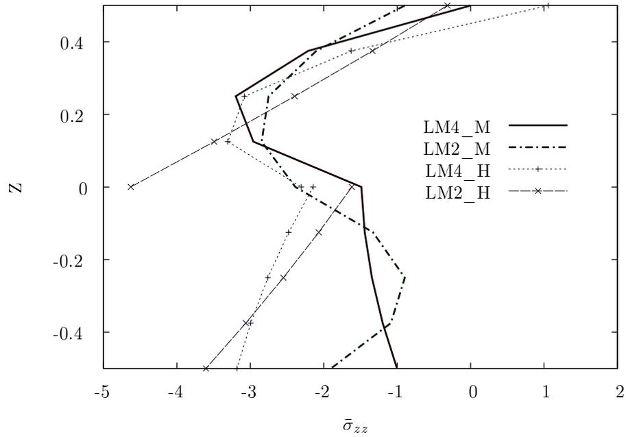
Figure 10:  $\bar{\sigma}_{zz}(L/2, 90^\circ)$  plot comparison for  $R/h = 500$ .
