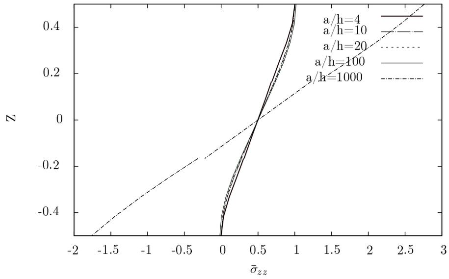
Figure 5:  $\bar{\sigma}_{zz}(a/2, b/2)$  (displacement formulation) distribution for different span to thickness ratio.
