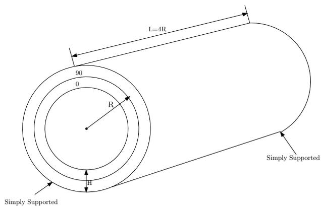
Figure 6: Laminated cylinder with stacking sequence  $[90^\circ/0^\circ]$ .
