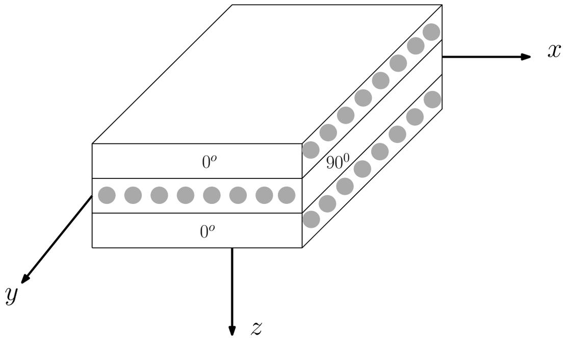
Figure 2: Laminated plate with stacking sequence  $[0^\circ/90^\circ/0^\circ]$ .
