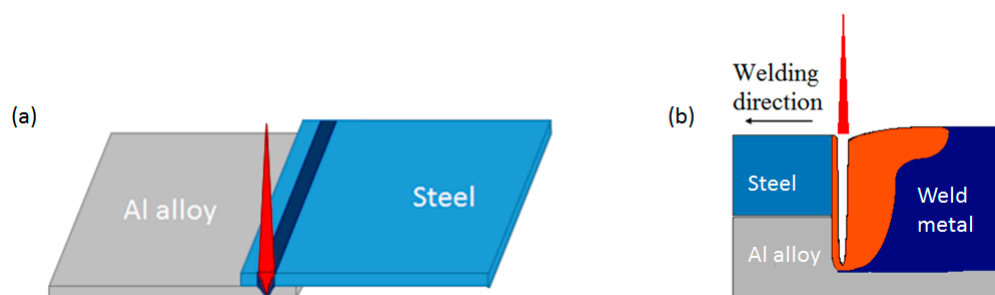
Figure 8. Laser welding with the keyhole mode: general view (a) and cross-section detail of the keyhole (b).
