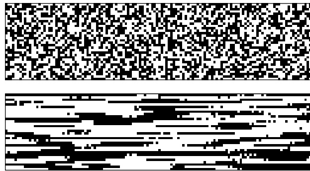
Fig. 2: An antipodal sensing matrix following standard CS (top) coupled with another antipodal sensing matrix generated as prescribed by the rakeness-based CS for ECG signals (bottom). Both matrices were generated with CR=4 . Note that white means -1 while black corresponds to +1 .
