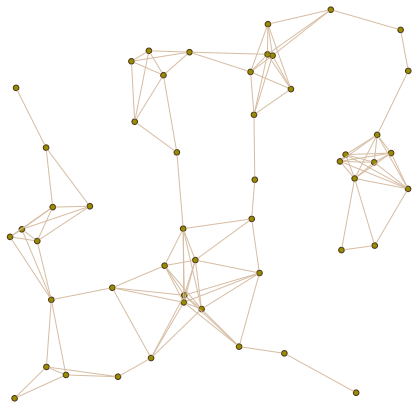
Fig. 2. Example of sensor node network with n = 50 and d_{th} = 0.2 . A connection between nodes indicates that they are related to the each other, i.e., their distance is smaller than d_{th} .
