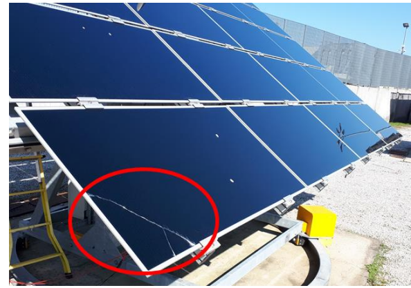
Figure 7. Detail of the broken module in plant E_{ts} (CdTe thin-film on an x-y tracking system).
