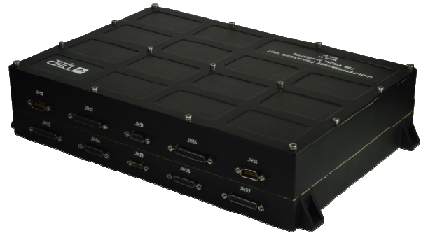
Figure 7: HPHC engineering model assembled in its cabinet
