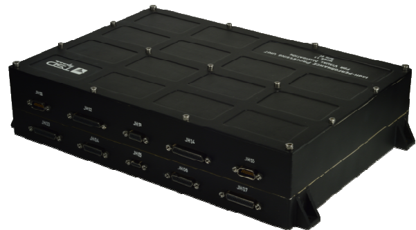
Figure 7: HPHC engineering model assembled in its cabinet
