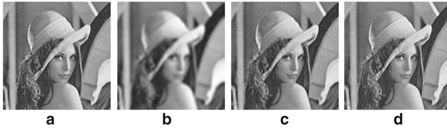
Fig. 13 Analysis of performance for Lena image deblurring: a original image, b acquired image, c FISTA reconstruction MSE (dB) = - 10.718 (after 1000 iterations), d 2-LMM-FISTA reconstruction MSE (dB) = - 13.3958 (after 1000 iterations)
