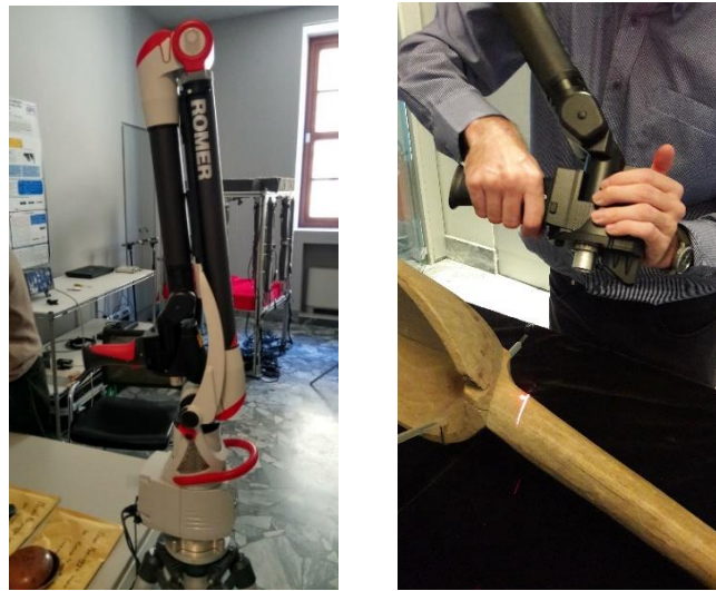
Fig. 2-3: On the left, the RS3 Integrated Scanner mounted on Romer Absolute Arm 7-Axis ‘SI’. On the right, an acquisition performed with the laser scanner.
