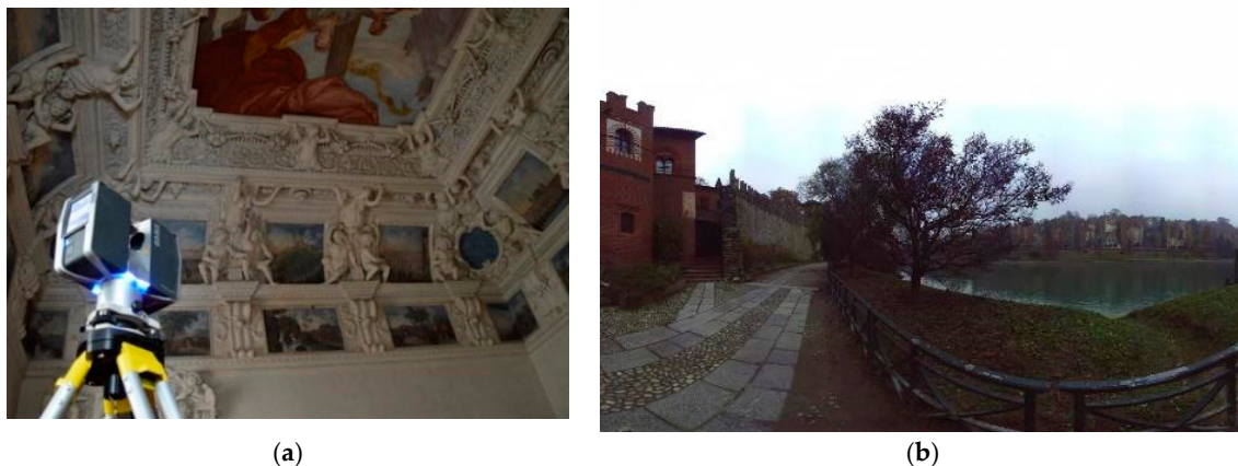
Figure 3. Terrestrial Laser Scanner (TLS) by FARO®: (a) The FARO® Focus 120 during the acquisition and (b) planimetric view of an outdoor coverage range of an X330 scanner.
