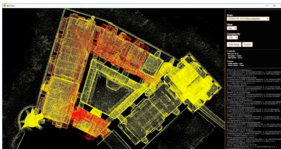
Figure 10. The desktop interface of the merge function in the GeoSLAM Hub software: in red, a single scan that is manually aligned, one at a time, to others, yellow. In the black box bottom right, the roto-translation matrix of each merged scan.
