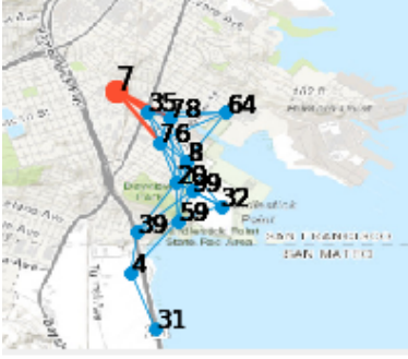
Fig. 2: Topology of interest: recharging site S (red dot) and zones Z (blue dots). Links identify sites/zones that are sufficiently close for a UAV-SC to fly from one to another in one TS.
