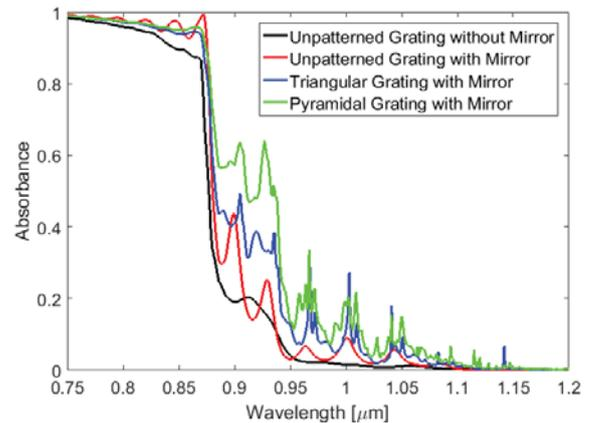
Fig. 6 Spectral dependence of the active region absorbance in planar cell without mirror, planar cell with mirror, cell with triangular grating (period=3  $\mu\text{m}$ , thickness=0.75  $\mu\text{m}$ ) and mirror, and cell with pyramidal grating (period=3  $\mu\text{m}$ , thickness=0.75  $\mu\text{m}$ ) and mirror. Average TE and TM polarization.
