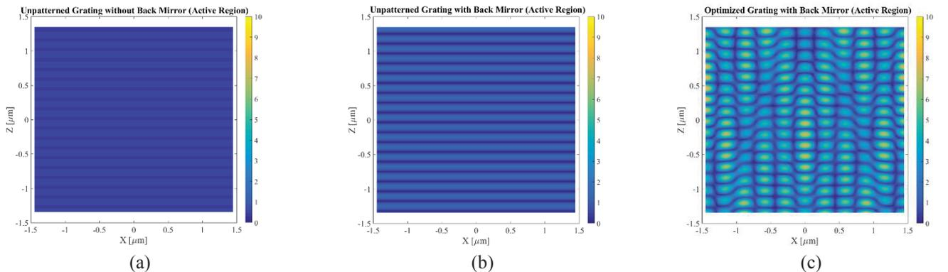
Fig. 2 Map of the calculated electrical field amplitude (TE excitation) at  $\lambda = 1000$  nm in the  $2.6 \mu\text{m}$  GaAs-QD photoactive region for the different configurations under study: (a) planar cell without mirror; (b) planar cell with mirror; (c) cell with rear side triangular grating ( $3 \mu\text{m}$  period and  $750$  nm height) and mirror.
