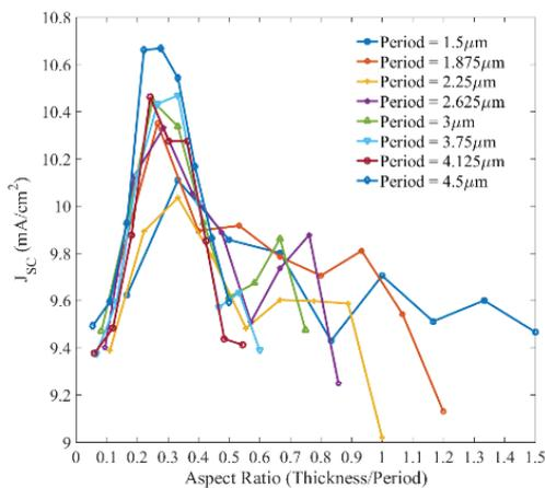
Fig. 4 Dependence of  $J_{sc}$  (0.75  $\mu\text{m}$  - 1.2  $\mu\text{m}$  wavelength range, TE polarization) as a function of the aspect ratio for different periods for the triangular grating configuration.
