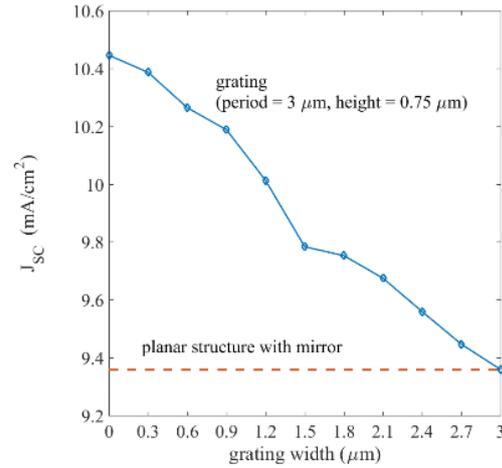
Fig. 5 Dependence of  $J_{sc}$  (0.75  $\mu\text{m}$  - 1.2  $\mu\text{m}$  wavelength range, TE polarization) as a function of the uni-periodic grating width: width=0 indicates the triangular grating, width=3  $\mu\text{m}$  identifies the unpatterned planar structure.
