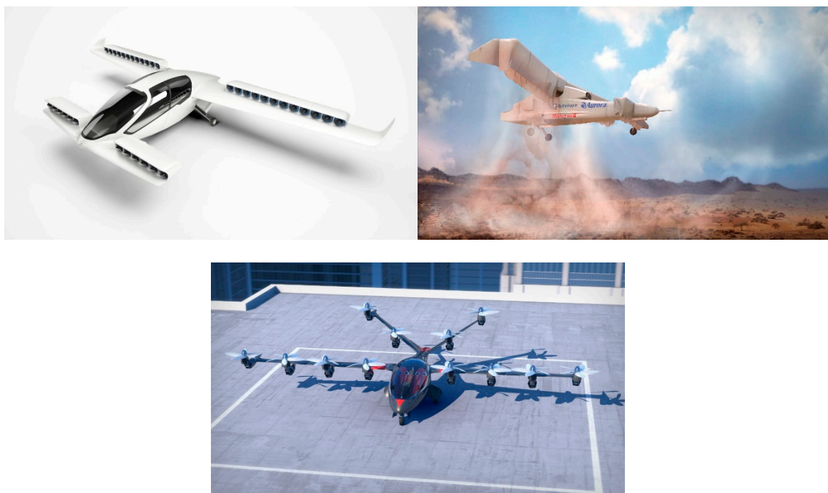
Figure 1. Vectored thrust electric vertical take-off and landing aircrafts (eVTOLs): Lilium Jet [13], Aurora Lightning Strike [23], Joby S2 [24].
