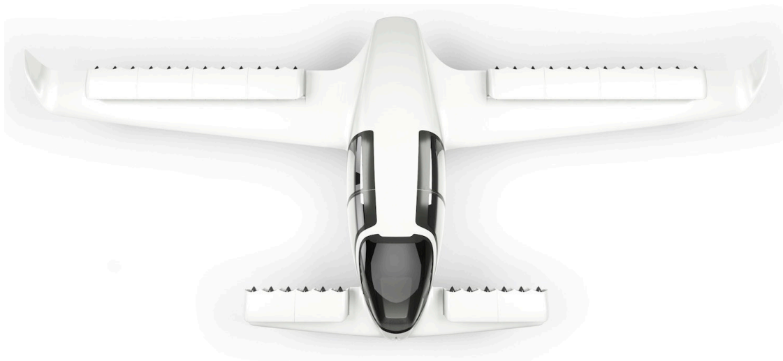
Figure 9. Lilium jet five-seater geometry.
