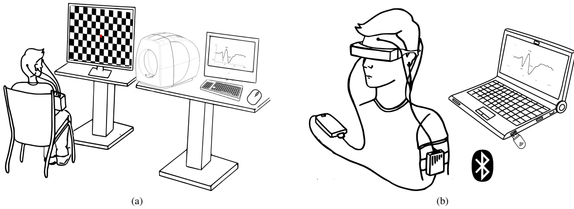
Fig. 2: Comparison between a traditional PR-VEP test (a) and a smart glasses stimulator-based PR-VEP test (b).
