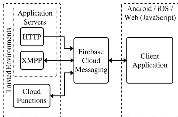
Fig. 3: Firebase Cloud Messaging general architecture
