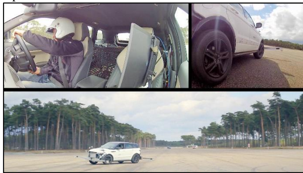
Figure 2. The four-wheel-drive electric vehicle demonstrator during a step steer test at the Lommel proving ground.
