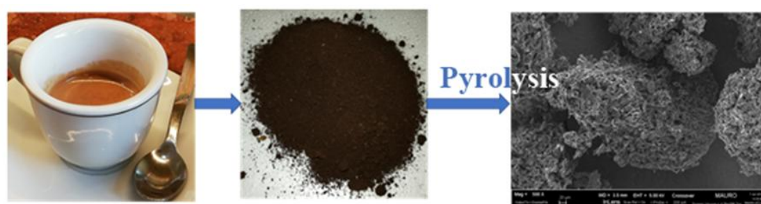
Figure 1. Conversion process of brewed coffee waste to carbon material.
