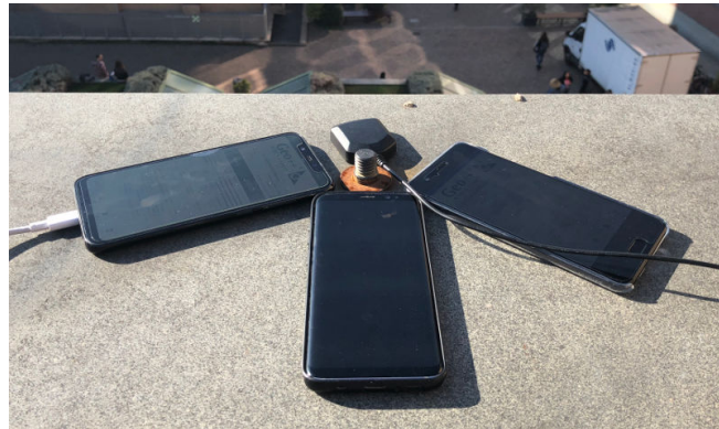
Figure 1. Setup of the data campaign carried out using smartphones. The screw indicates the georeferenced known point.
