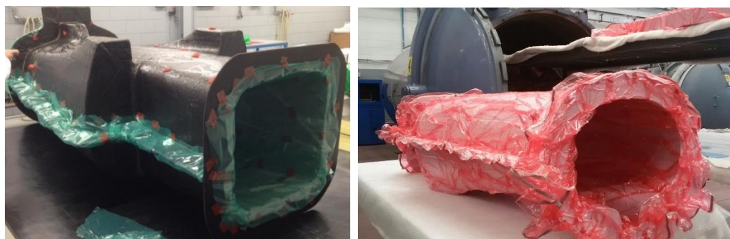
Figure 12. First lamination: Release film ( left ) and vacuum bag ( right ) on the female central mold.
