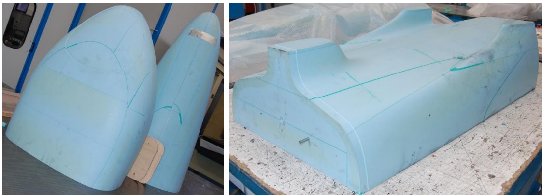
Figure 11. Male resin molds; front and rear end (left), and central part (right).
