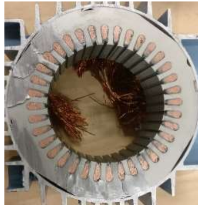
Fig. 1. Cut-section of the commercial induction motor stator.
