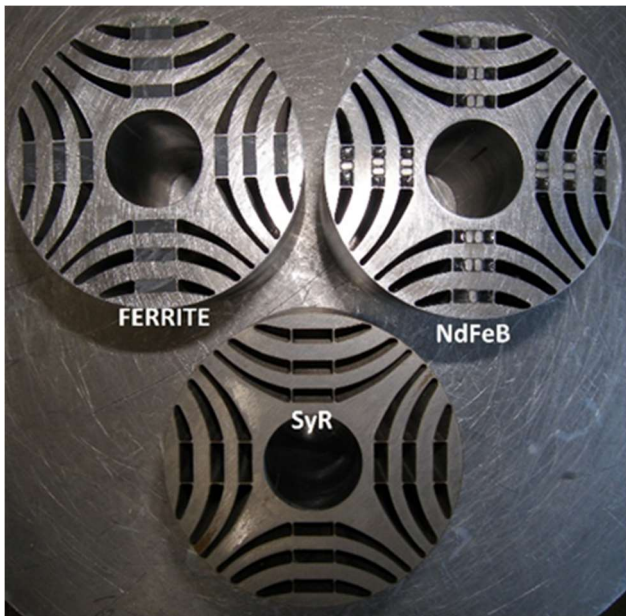
Fig. 5. Picture of the three prototype rotors assembled.
