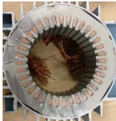
Fig. 1. Cut-section of the commercial induction motor stator.
