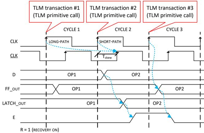
Fig. 7. Mapping of RTL waveforms to TLM transactions for the Razor sensor.
