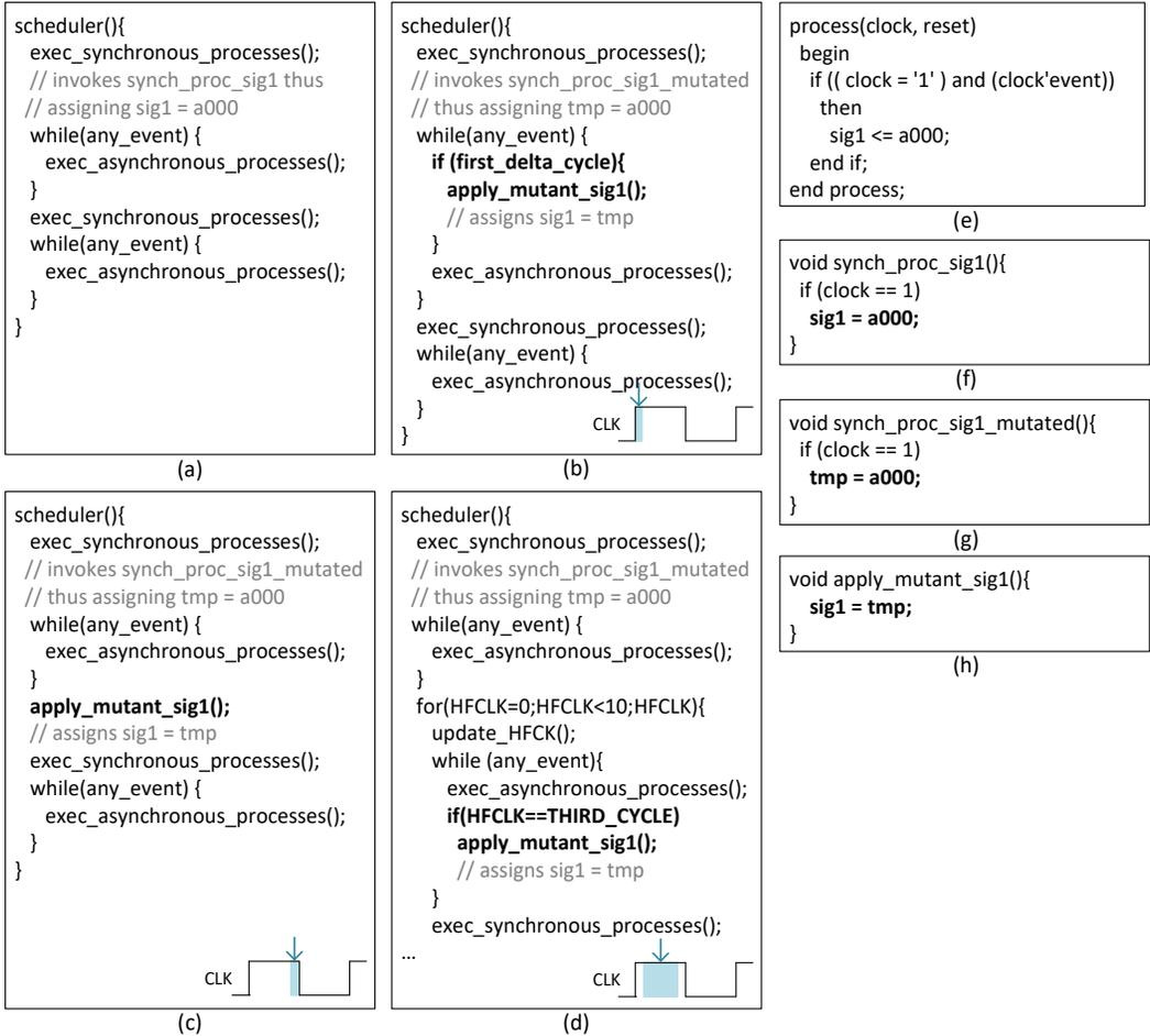
Fig. 9. The proposed mutants for the TLM model: high-level representation of the TLM scheduling without mutants (a), a *minimum delay* mutant example (b), a *maximum delay* example (c), and an example of delta delay mutant (d). The snapshots of code apply delays to the assignment `sig1 = a000`, for which the figure shows the original VHDL code (e), the corresponding C function (f), and the effect of mutant injection (g-h).
