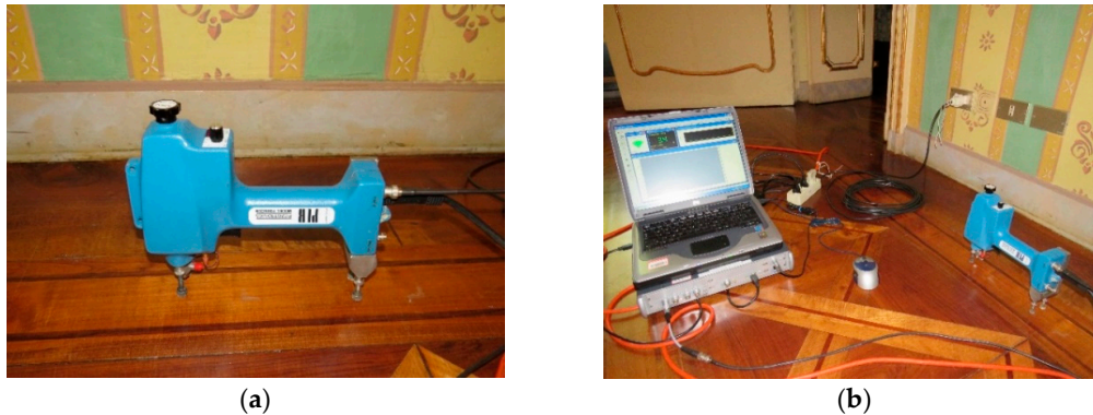
Figure 4. (a) The electric impact hammer; (b) the LMS Pimento multi-channel signal analyzer.
