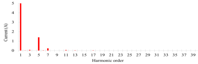
Fig. 5: Spectral analysis of current of converter #7B. The 50 Hz component (truncated in the graph) is 15.4 A
