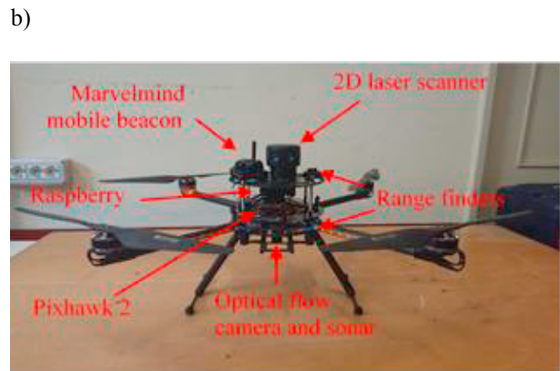
Fig 2. a) hardware architecture, b) drone platform and sensors
