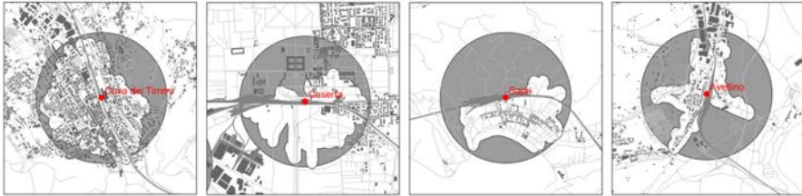
Fig.2 Examples of calculated pedestrian catchment areas (CA) for some station areas of Campania region rail network
