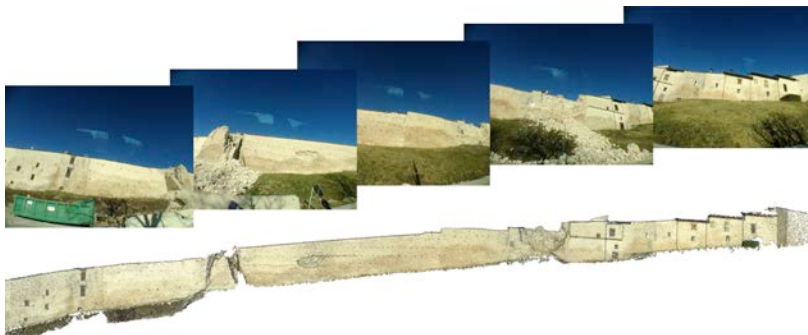
Fig. 2 Frames of Norcia's image sequence and 3D point cloud frontal view
