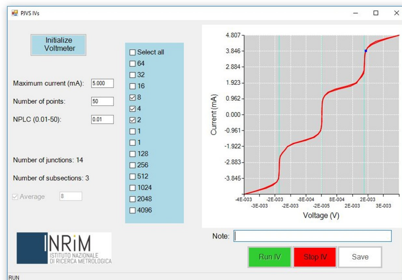
Fig 6. PJVS IV-characteristics GUI. The graph displays the averaged current-voltage characteristics of fourteen Josephson junctions subdivided in three consecutive sub-arrays.
