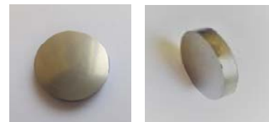
Fig. 2. Sintered Ti 2 AlN MAX phases samples
