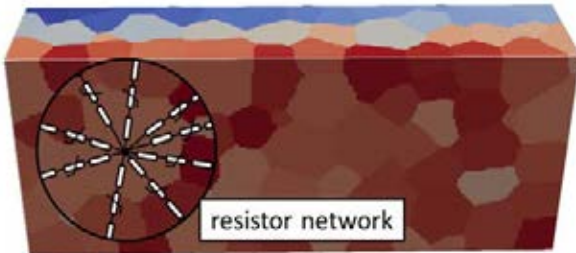
Fig. 7. 3D model of the ZnO microstructure as a basis for a resistor network.
