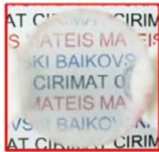
Fig. 3. Small alumina sample size ( \varnothing 20mm Thickness 0.88mm) RIT > 70%
