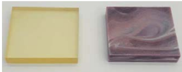
Fig. 2. Fresnoite glass (left) and glass-ceramic (right)
