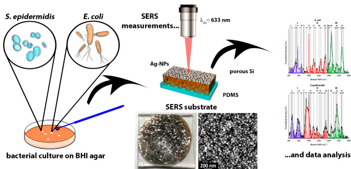
Figure 1. Scheme of the surface enhanced Raman spectroscopy (SERS) analysis of E. coli and S. epidermidis grown on brain heart infusion (BHI) agar and collected after different times of culture.
