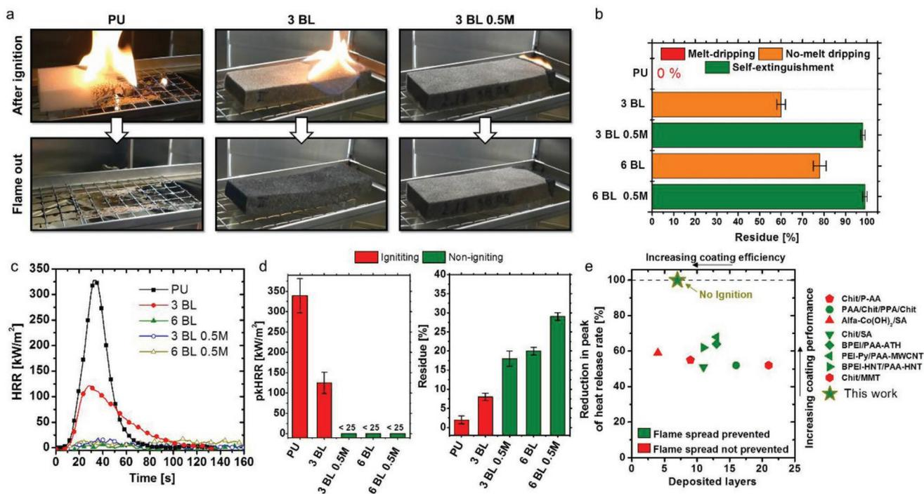
**Figure 4.** Flame retardant characterization of untreated and LbL treated foams: a) snapshots from flammability tests, b) average residues after flammability tests, c) heat release rate versus time plots, d) average peak of heat release rate and final residue, and e) flame retardant performance comparison with previously reported materials.
