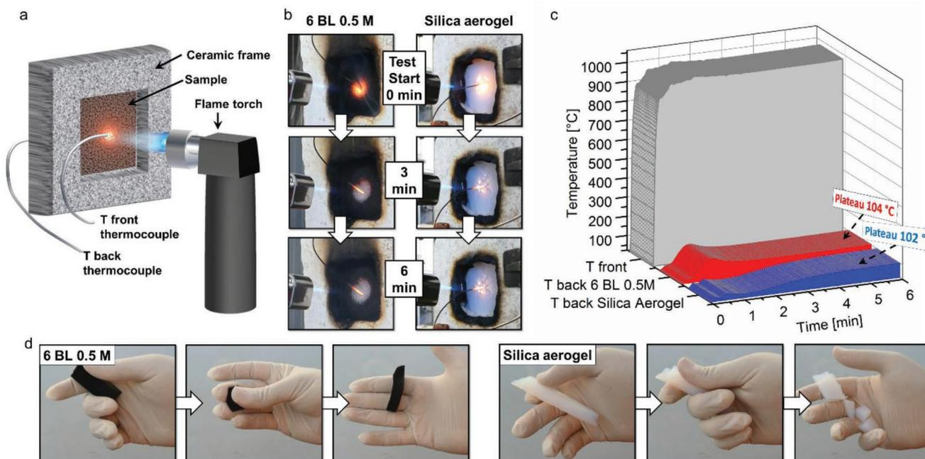
**Figure 6.** Flame penetration tests: a) schematic representation of the layout adopted for the test, b) digital pictures of the 6 BL 0.5M and silica aerogel front surface during the test, and c) front and back side temperatures as a function of time for 6 BL 0.5M and silica aerogel. d) simple bending test performed on 6 BL 0.5M foam and silica aerogel.
