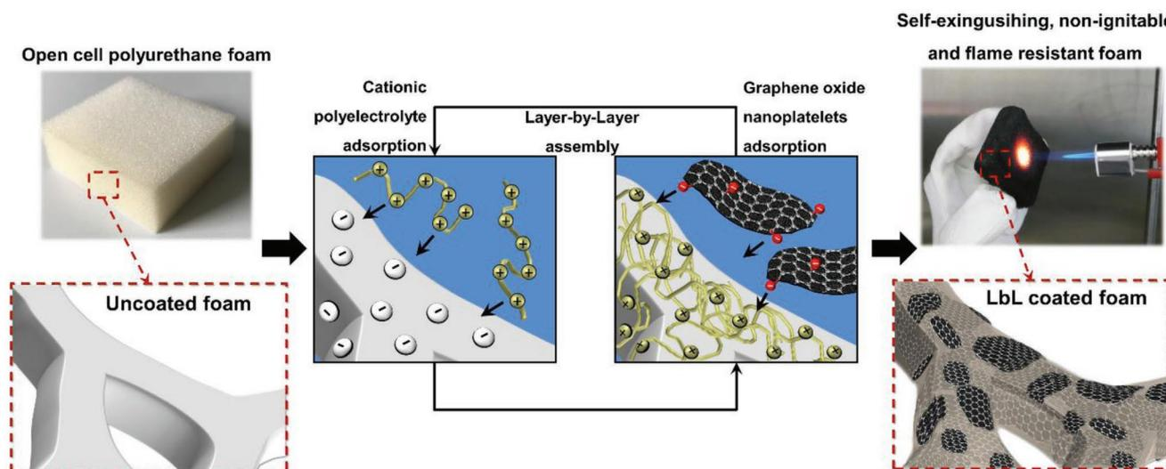
**Figure 1.** Schematic representation of the deposited LbL assembly. PU foams are alternatively dipped in cationic polyelectrolyte solution and negative graphene oxide nanoplatelets suspension. Each cycle deposits a bi-layer (BL), the process is repeated in order to deposit 3BL and 6BL.
