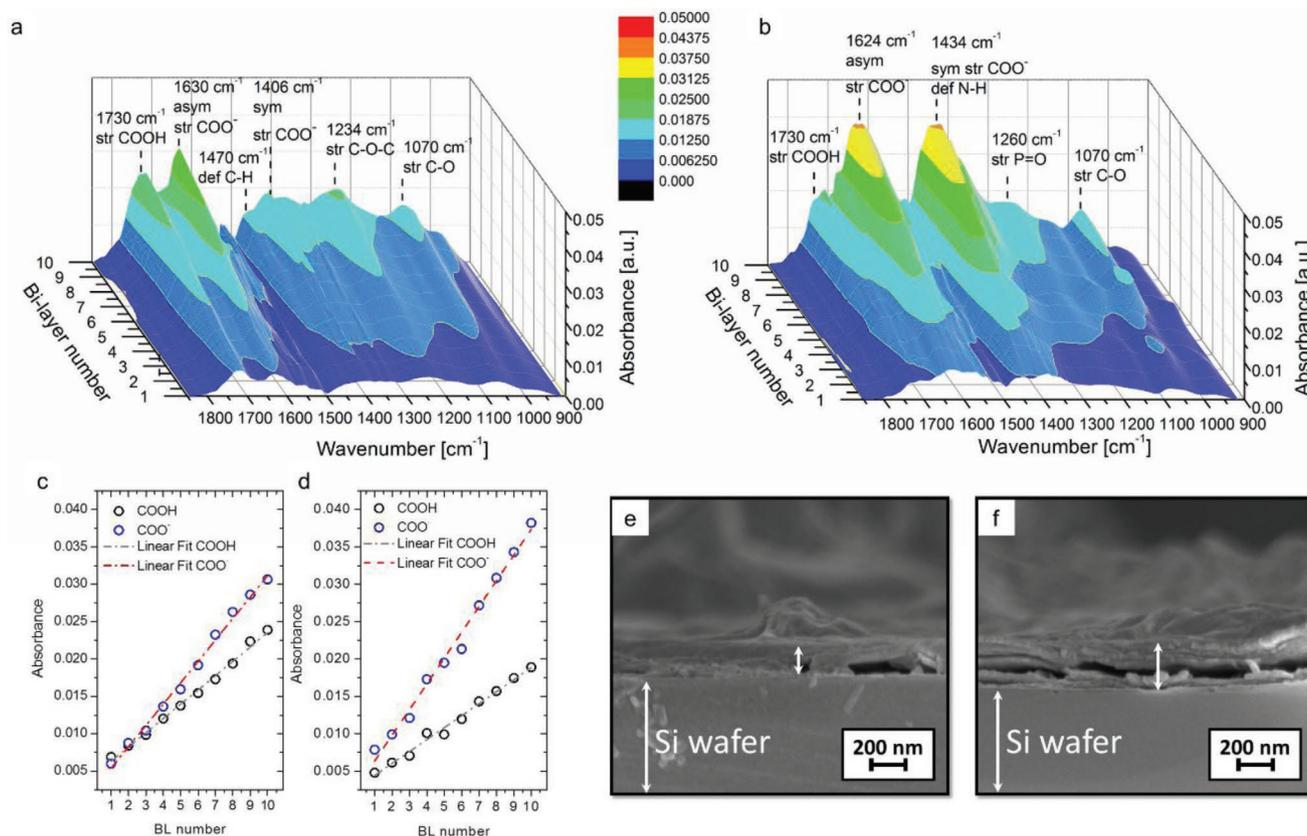
**Figure 2.** Characterization of the build-up of PDAC/GO at 0 a,c,e) and 0.5M b,d,f) APD on model Si substrate: a,b) FT-IR spectra in the 1850–900  $\text{cm}^{-1}$  region during LbL growth; c,d) evolution of the signals ascribed to COOH and  $\text{COO}^-$  as function of bilayer number and e,f) FE-SEM micrographs of 10 BL cross-section on Si wafer.
