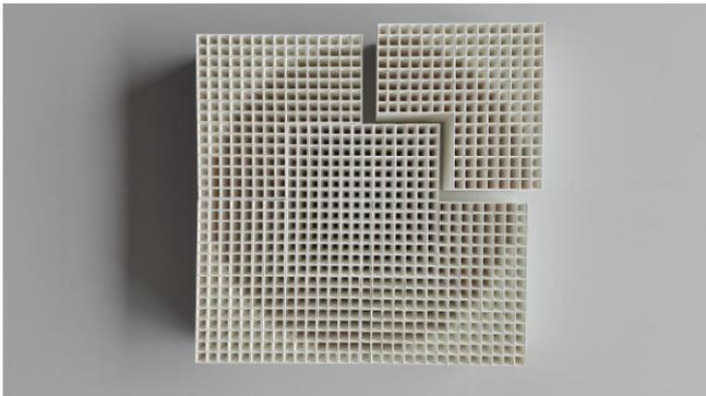
**Figure 2:** 3D-Printed prototype of the dielectric transmitarray using FDM technique.
