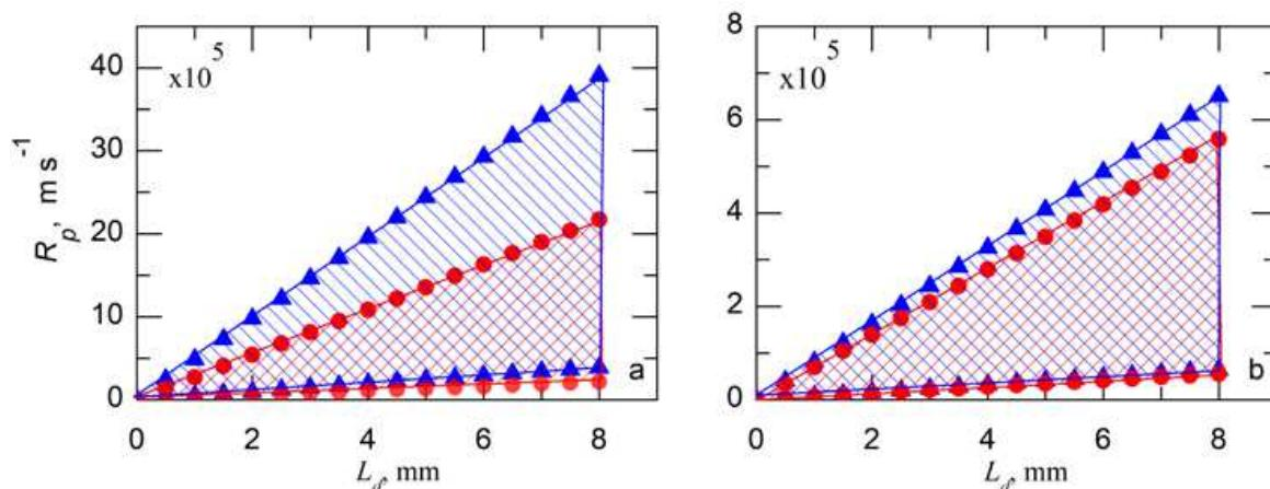
**Fig. 4 Uncertainty in the value of  $R_p$  as function of the dried layer thickness  $L_d$ , due to the uncertainty on  $\tau$ . The range 1.2–3.8 was considered for  $\tau$ . (a) conventional freezing, and (b) VISF. ●: Values calculated using Eq. 1, in which the pore dimension  $D_p$  was obtained by the image segmentation approach; ▲: Values calculated using Eq. 1, in which the pore dimension  $D_p$  was obtained by the traditional manual approach.**
