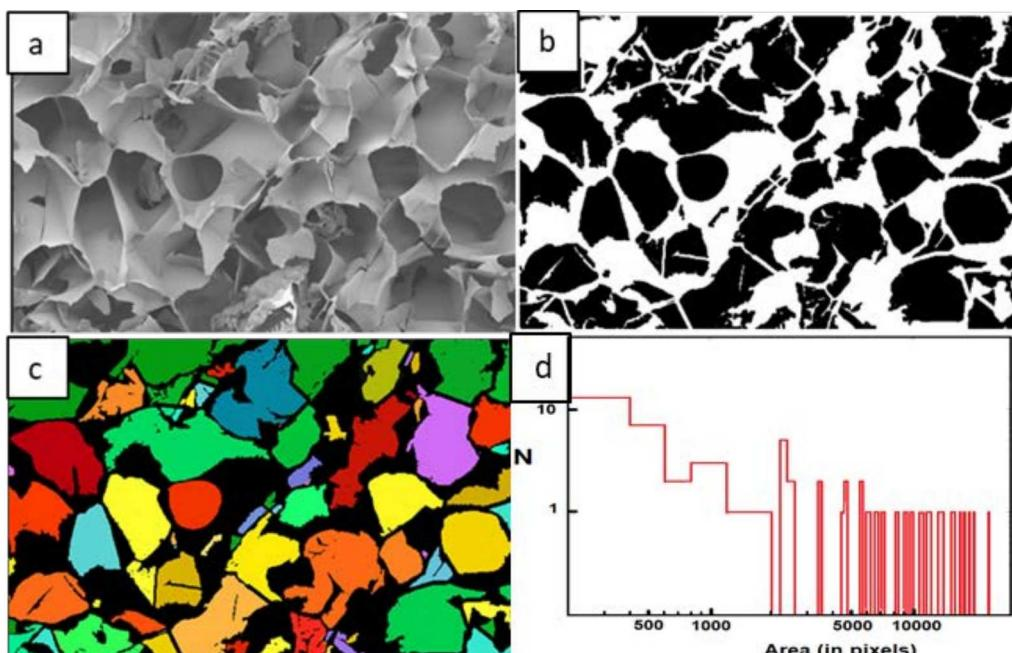
*Fig. 2 (a) SEM and (b) binary images corresponding to mannitol 5% w/w, freeze dried using VISF. (c) Segmentation of the original SEM image, where the domains are represented by different colors. (d) Distribution of the super-pixels (in logarithmic scales), obtained by counting them according to their area (in pixels).*
