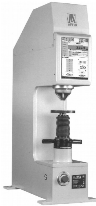
FIGURE 4. AFFRI ® LD 3000 AF hardness testing machine.
