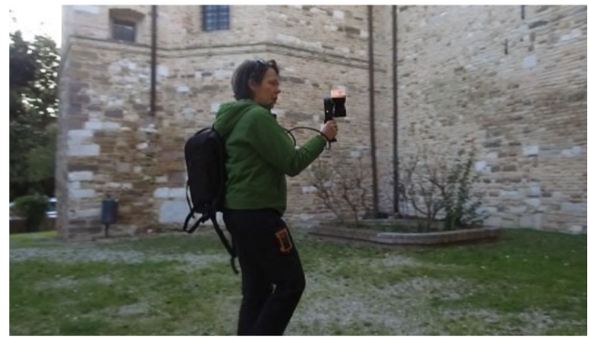
Fig. 1 The ZEB-REVO system with the rotating ranging head, tested by Geomatics Lab for Cultural Heritage, PoliTo, in 2017 in San Severino Marche (MC)
