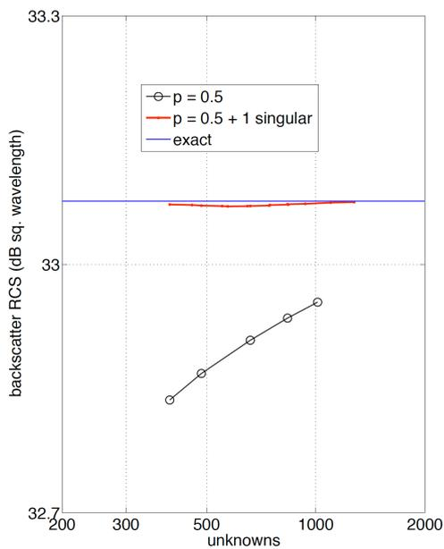
Fig. 8. Backscatter RCS for a disk with  $ka = 4$ , for a range of mesh sizes. Numerical results based on polynomial basis functions ( $p = 0.5$ ) and a mixture of polynomial and singular basis functions ( $p = 0.5 + 1$  singular) is compared to the exact solution.
