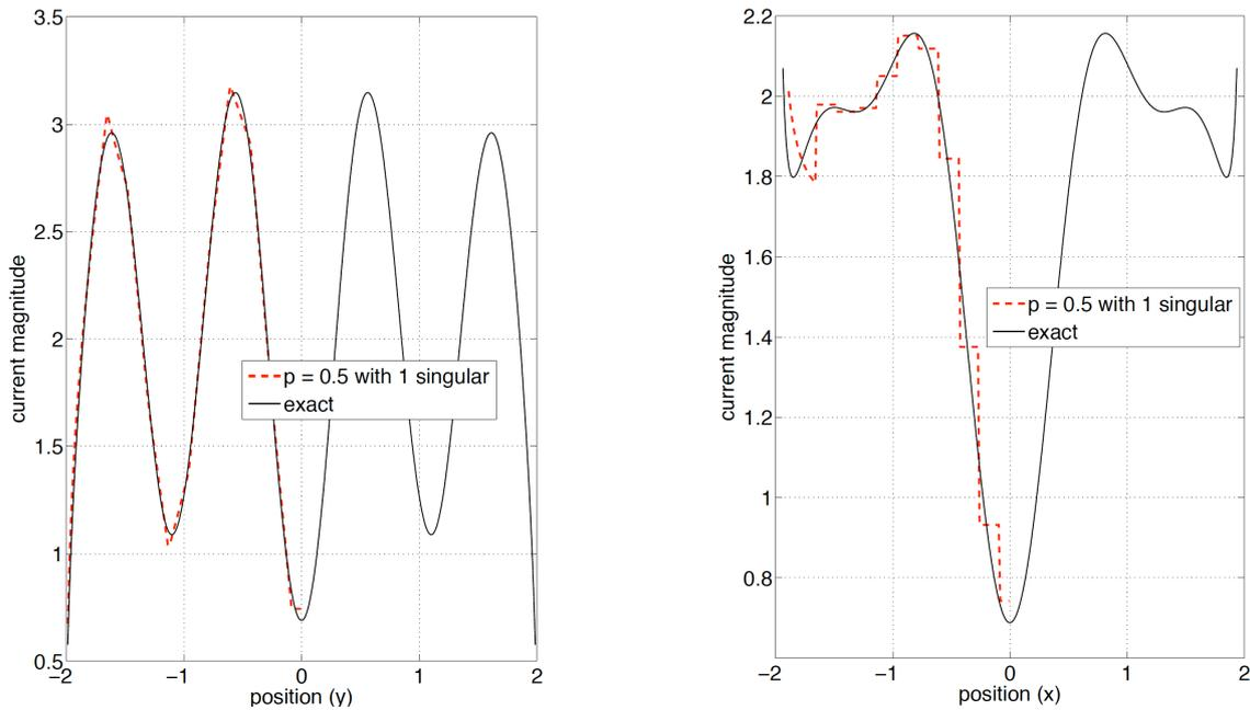
Fig. 7. The figures show the co-polarized current induced on disk with  $ka = 4\pi$  by a normally incident plane wave with unity magnitude  $H$ -field. The numerical result incorporating singular basis functions in the edge cells for a 341-cell mesh is shown over half the range, for a cut through the disk center along the  $y$ -axis (at top) and  $x$ -axis (at bottom).
