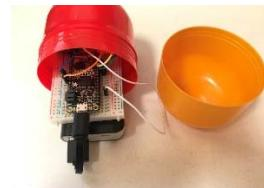
Fig. 5. Configuration of one of the used transmitters for star-topology network measurements. The prototypal transmitter is powered with a power bank connected to the electronic board through a USB cable. The antenna is inside the plastic enclosure.
