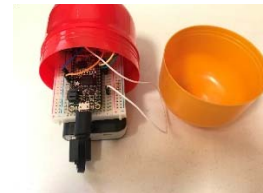
Fig. 5. Configuration of one of the used transmitters for star-topology network measurements. The prototypal transmitter is powered with a power bank connected to the electronic board through a USB cable. The antenna is inside the plastic enclosure.
