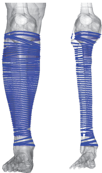
Fig. A3. Lower part of the LLMS model: in blue the sections where the bending moment on the tibia was measured.
