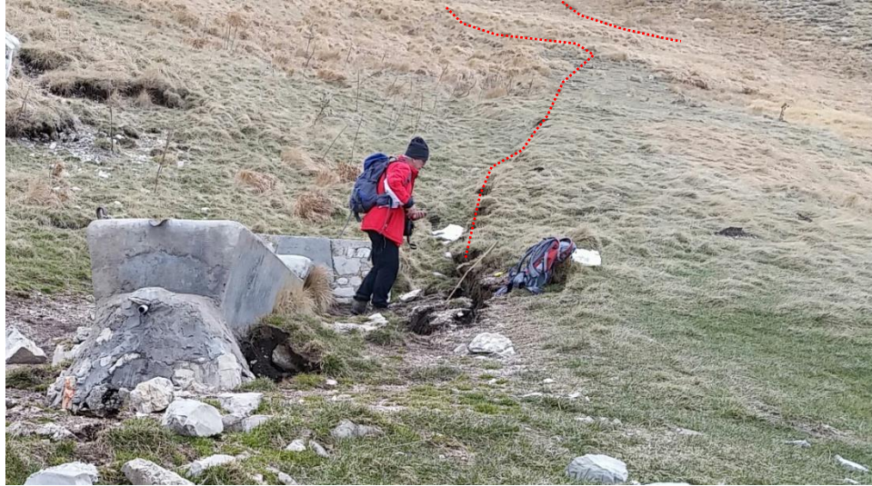
Figure 2.16. Fault trace on the south face of Mt. Vettore, where the fault has ruptured along the path of buried polyethylene pipe supplying the pictured spring. Rupture partially hidden by long grass. Offset measured at 45 to 65cm. August offset data nearby is 0 to 15cm. Trace(s) above the spring indicated in red. Lat = 42.80474, Long = 13.26441.
