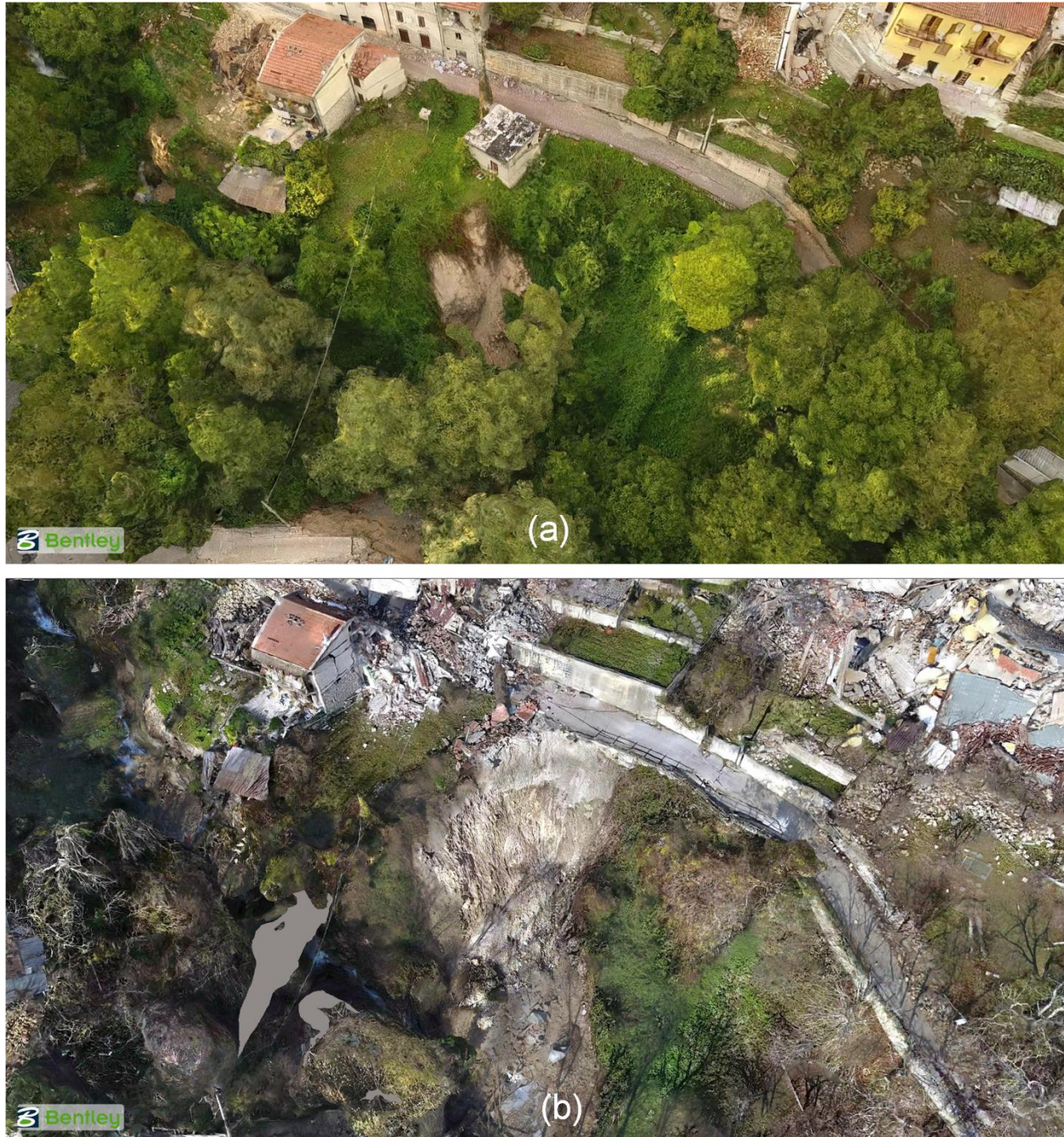
Figure 4.26. 3D model comparison of the landslide near the head of the gulley in Pescara del Tronto between September 2016 (a) and December 2016 (b).
