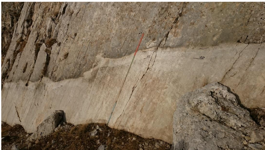
Figure 2.13. Fault slip measurements showing multi-epoch offsets from August 2016 (upper white band, 16 cm) and October 2016 (130 cm) events. Lat = 42.81724, Long = 13.25449.
