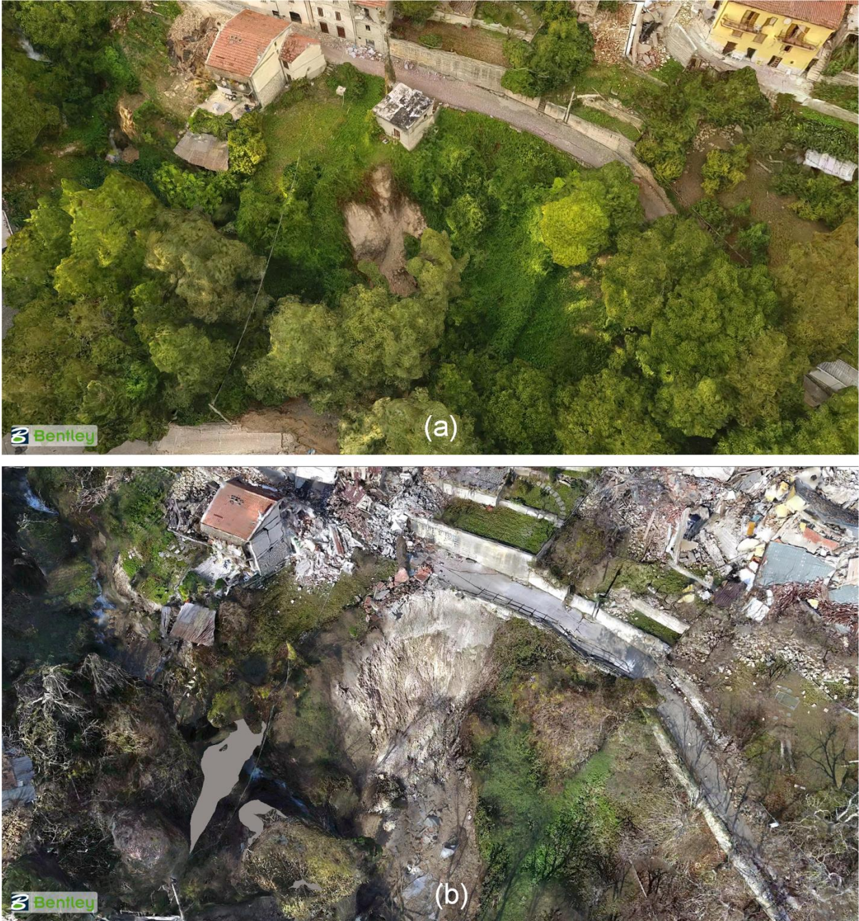
Figure 4.26. 3D model comparison of the landslide near the head of the gully in Pescara del Tronto between September 2016 (a) and December 2016 (b).
