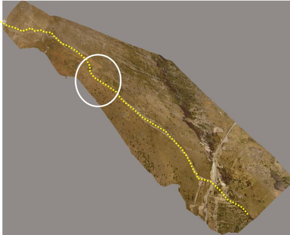
Figure 2.9. 3D digital terrain model from merged SfM and LiDAR data of the Mt Vettore fault on the southern flank of the Mt Vettore Massif. Approximate main fault trace indicated in yellow. Looking from the west to the east. The upper left of the image is the top of the slope. Area of soft sediments where the fault trace breaks into several (4 – 6) small scarps is indicated in white.
