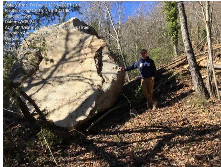
Figure 4.48. Last boulder fragment (4 meter) from rockfall near road at base of slope. Also pictured are freshly toppled trees from the boulder’s roll to its final position.
