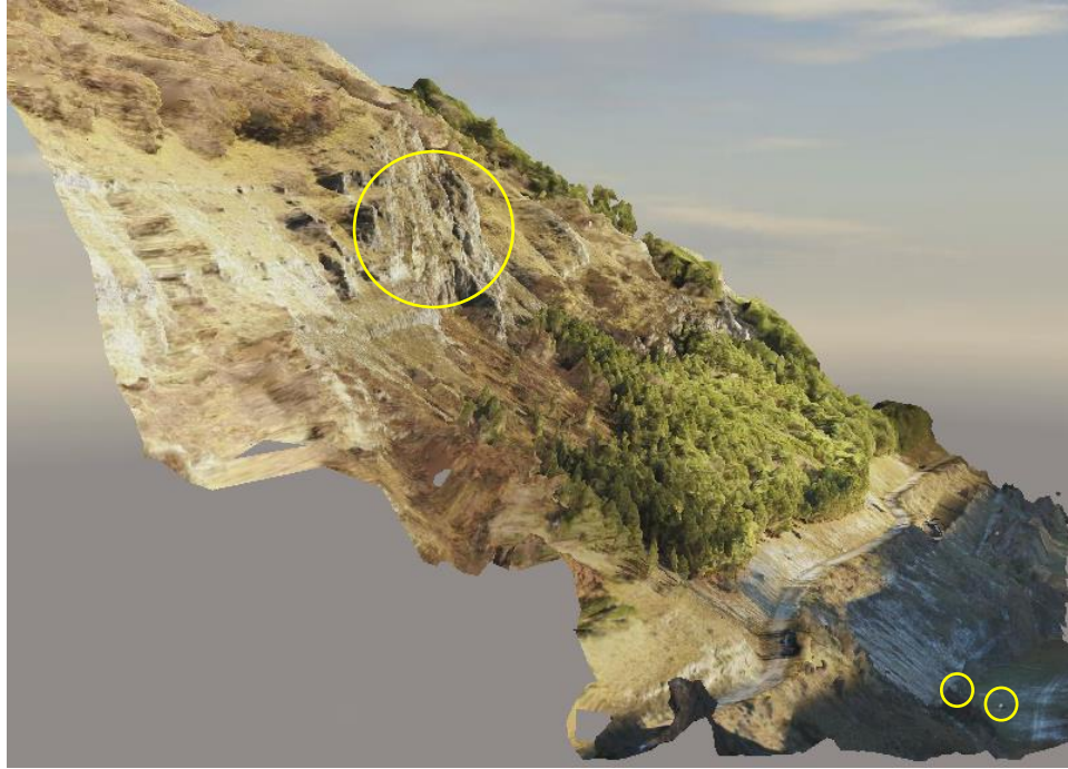
Figure 4.56. Pescia rockfall site 9a 3D SfM model from UAV data. Rock source and 2.5 meter boulders circled in yellow.
