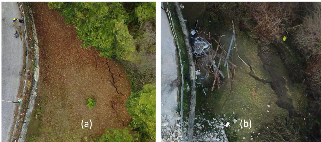
Figure 4.35. 3D model screenshots showing cracking from a shallow landslide (a) during the September GEER reconnaissance, and (b) during the December GEER reconnaissance.
