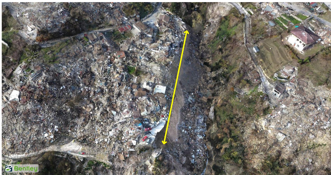
Figure 4.25. 3D SfM model view of scarp linearity behind failed lower retaining wall in Pescara del Tronto.
