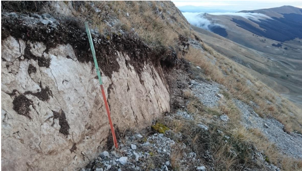
Figure 2.12. Fault offset measurements showing relative offset of August 2016 (0 cm) and October 2016 (70 cm) events on the lower or “western” fault trace in Figure 2.10 (shown in white). Lat = 42.812901, Long = 13.24626.
