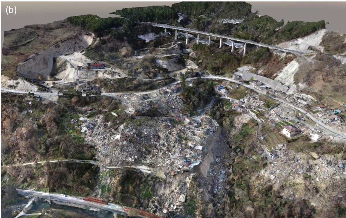
Figure 6.58. 3D-model overview of Pescara del Tronto from a common perspective (a) after the 24 August earthquake, and (b) after the October events.
