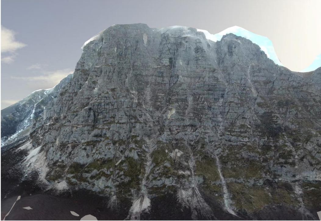
Figure 4.11. Screenshot of Monte Bove SfM meshed 3D model. Note the missing summit of the mountain in the model due to insufficient UAV imagery
