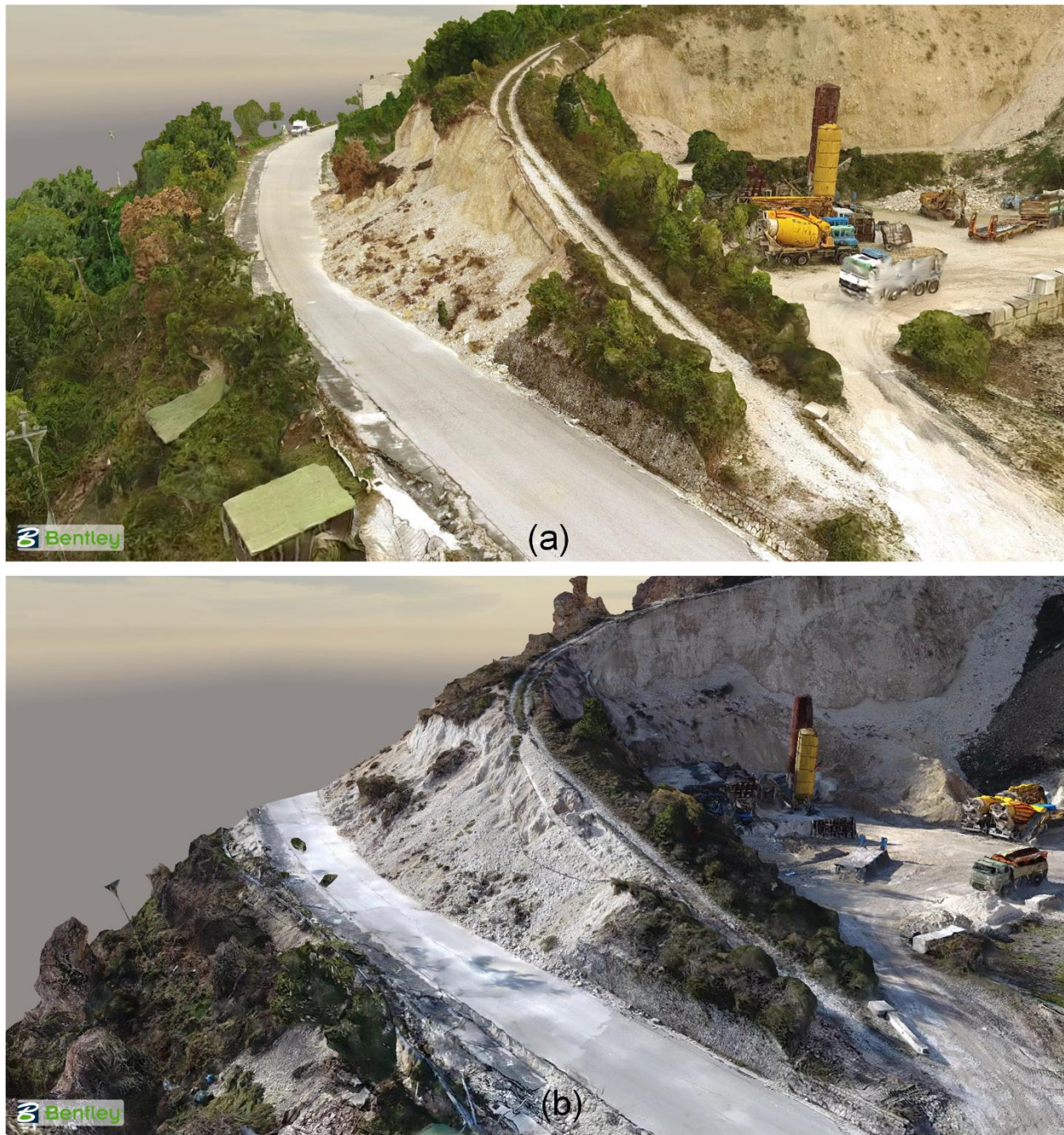
Figure 4.28. 3D model comparison of the landslide near the gravel pit in Pescara del Tronto between September 2016 (a) and December 2016 (b).
