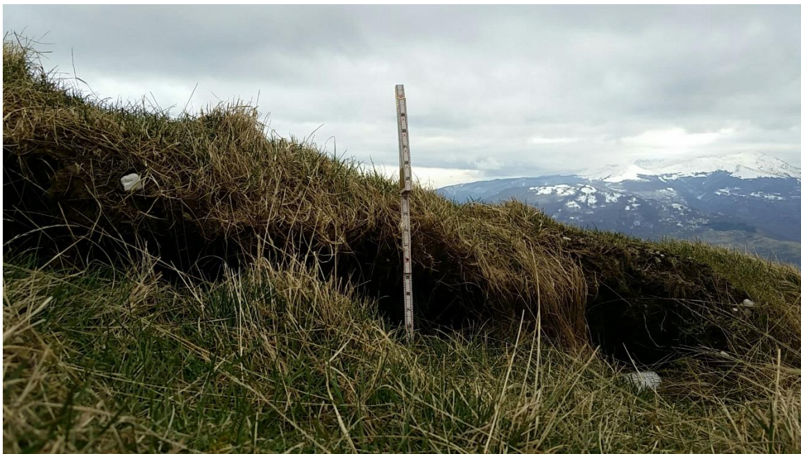
Figure 2.17. Fault offset measurement of one of several (4 to 6) small traces on the south face of Mt. Vettore in the area indicated in white in Figure 2.9. In this area surface soils are thick and ductile. Offset measured at 8 to 52cm on each trace. August offsets were 0 cm. Lat = 42.80483, Long = 13.26443.
