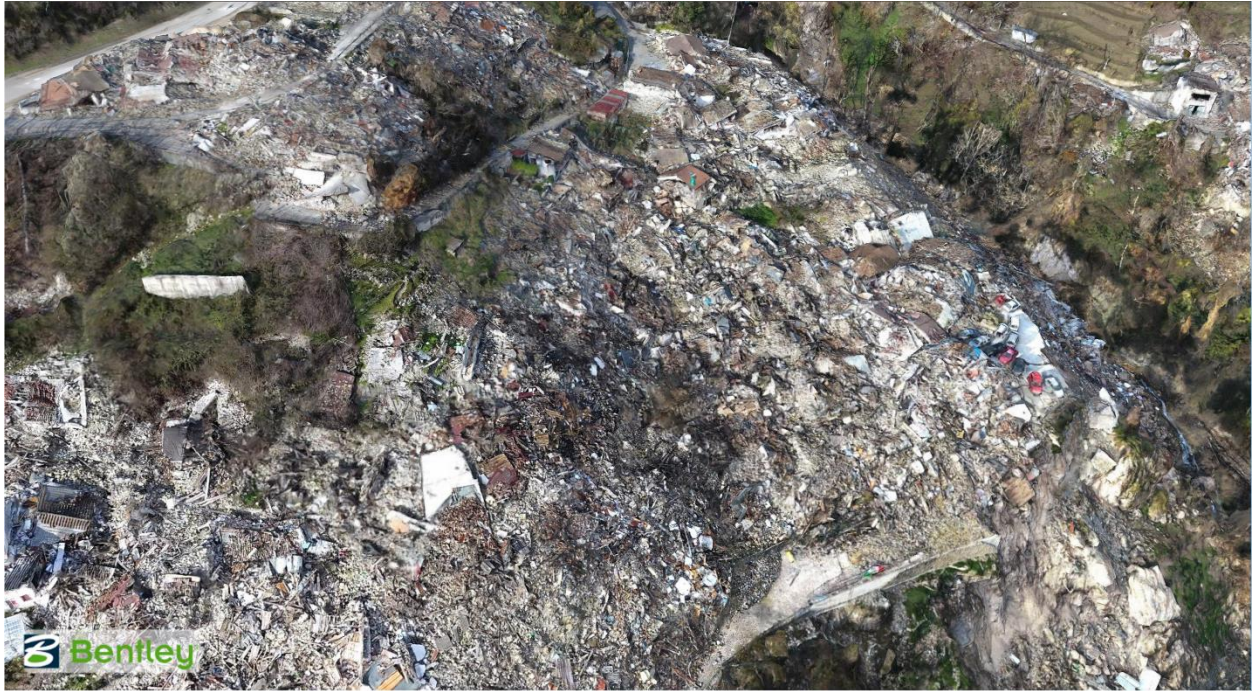
Figure 4.14. 3D SfM model of main damaged building area overlying talus deposits (Location 3a).
