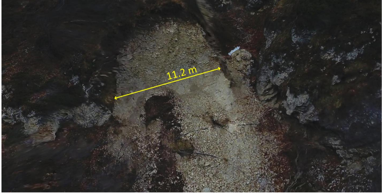
Figure 4.42. 3D model of the source of the Valle di Panico rockfall, located 90 meters above the mountain road.
