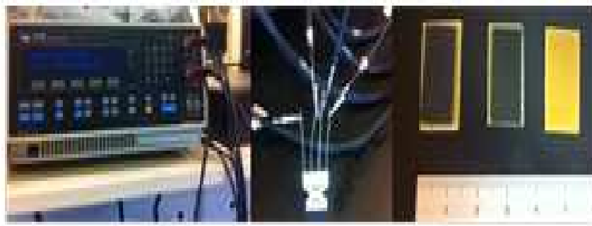
Figure 13. Four probe method: Solartron SI 1260 (left), sample holder (center), sample on FR4 2×1 cm (right).
