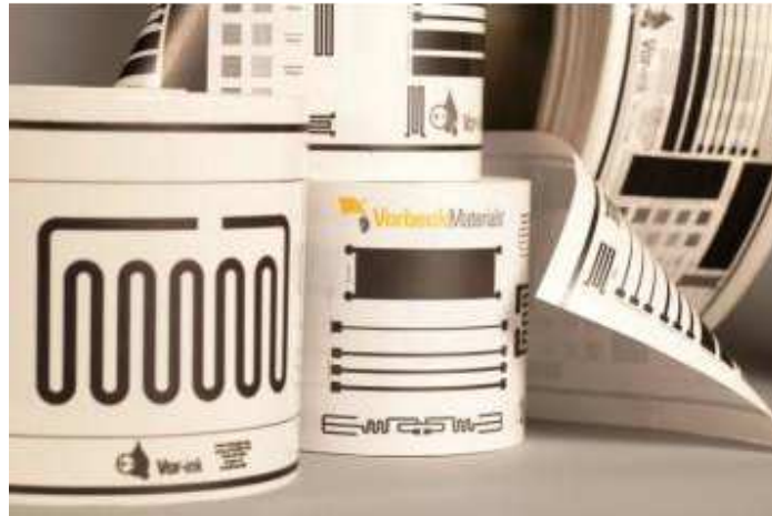
Figure 6. Graphene inks used for printed electronics. www.graphene-info.com/taxonomy/term/63/all
