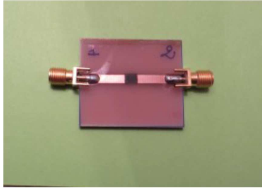
Figure 14. Microstrip line with graphene thin film deposition in the gap.
