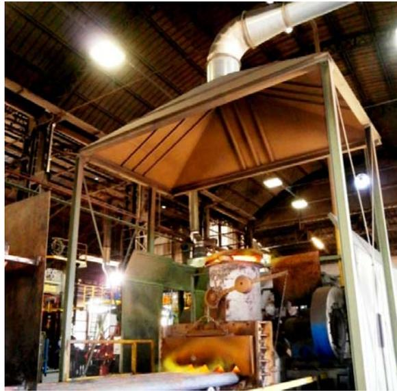
**Figure 3.** Methane oven in the factory for the heating of steel bars with extractor hood
