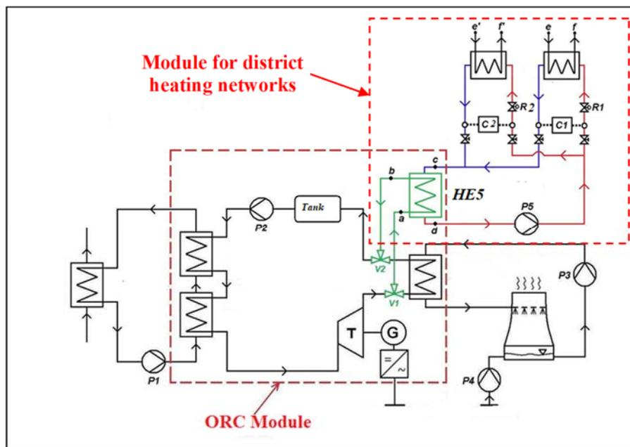
**Figure 9.** Scheme of the ORC module with additional thermal recovery for district heating networks. Legend of symbols: HE5 organic fluid-water heat exchanger; HE6, HE7 heat exchanger for district heating networks; P5 water circulation pump; V1, V2 three-way valves; C1, C2 energy meters; R1, R2 control valves.
