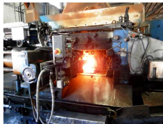
Figure 2. The exit door of the oven where the steel bars are cut by means of shears system.
