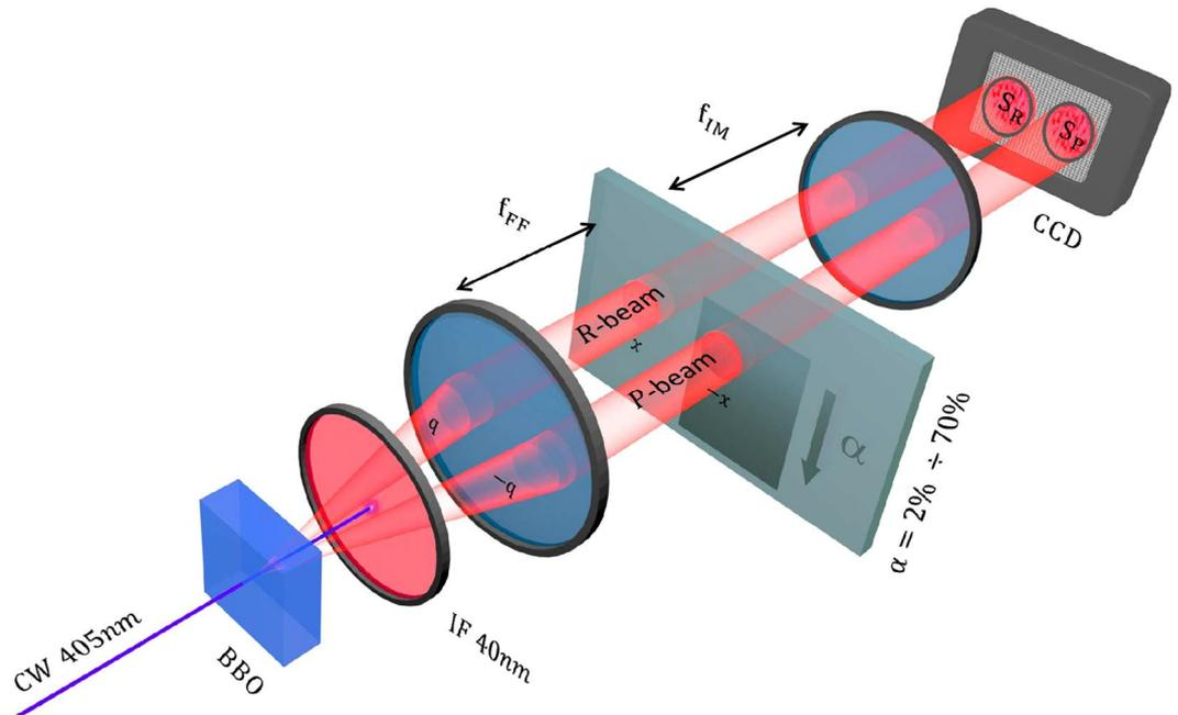
**Figure 2.** Scheme of our experimental set-up. In the BBO crystal two beams with perfect correlation in the photon number (TWB state) are generated. The probe beam passes through the sample and is then detected in the  $S_p$  region of the CCD, on the contrary the reference beam goes directly to  $S_R$ , without interacting with the sample. A detailed description of the optical components can be found in the text.
