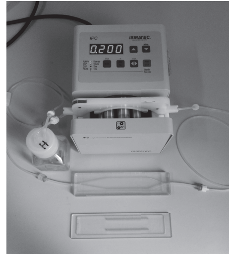
FIGURE 1: Assembled laminar flow bioreactor (LFB). Bioreactor is composed by a mixing chamber filled with a complete culture media with 5% of Dextran, a cell culture chamber, and a peristaltic pump. All the components were connected in a closed loop and put in an incubator to preserve temperature (37°C) and CO 2 concentration in air (5%).
