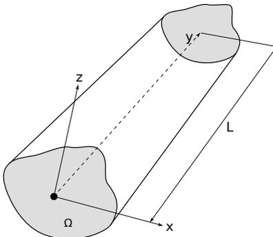
**Figure 1:** Coordinate system for the 1D beam model
