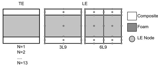
**Figure 9:** Cross-section configurations for the sandwich beam
